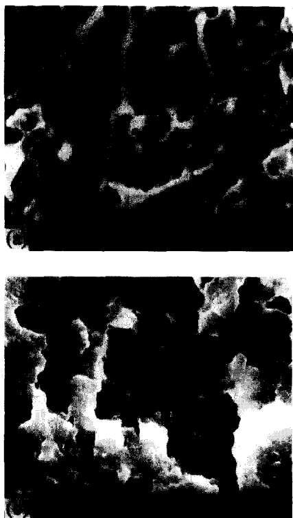
Figure 6 Fractographs for a brittle PVC/NBR blend with the pseudonetwork morphology taken in (a) the region A and (b) the region B
